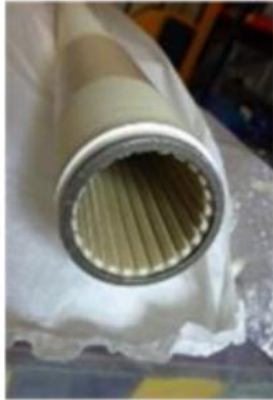
Cr2O3 coated alumina tube (MKI)
