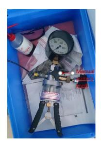
Figure 4. Manual pump used to pressurise the  $\mu\text{OHPs}$
