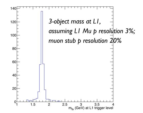
Start from LI\_TripleMu0 40 kHz @ 5E34 Track trigger & pT>2 GeV => a factor of 1/5 Invariant mass < 3 GeV => a factor of 1/20 => 400 Hz at 5E34
