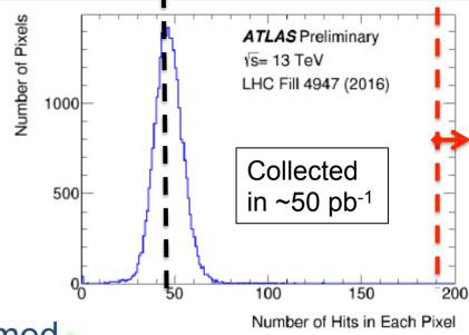
→bit flip on single pixel threshold (TDAQ) seems to be the main cause.
