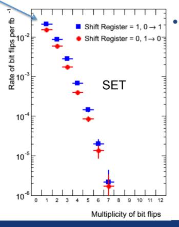
Differences between the opposite transition: "chip to chip" process variations, tuning and particle flow differences.
