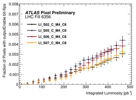
Shown for four different FE-I4 front ends placed on various IBL 3D modules as a function of the integrated luminosity of the fill.
