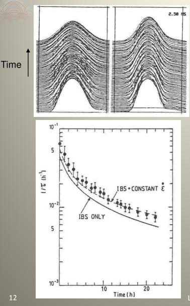
Bunch lengthening with time for a strong proton bunch (left) and a weak antiproton bunch (right).
