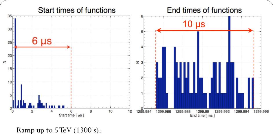
Collimators in different locations start together within  $6 \ \mu s$ . End times of profiles within  $10 \ \mu s$ .
