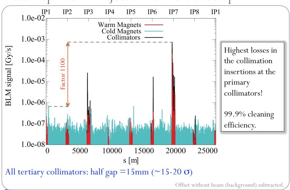
Loss Map Beam 1 Injection for Partial Setup
