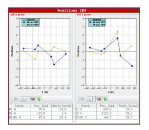
$\Rightarrow$  (Large) IP transverse offset remaining. Difficult to correct using closed orbit bumps because of aperture limitations.
