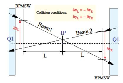
$\Rightarrow$  Correcting the offsets to align beams based on BPM measurements with local closed orbit bumps was sufficient to establish collisions at the four IPs.
