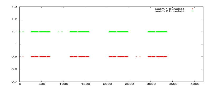
Filling scheme for 720 bunches per beam, extra bunches for IP2
