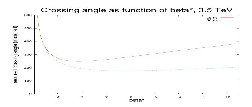
Total crossing angle required for 3.5 TeV (for 'sufficient' separation)
