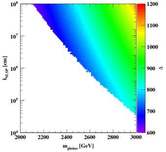
Gluino mass is pushed above 3 TeV for singlino lifetimes leading to displaced vertices
