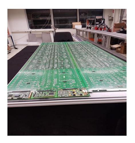
**DIF** sends DAQ commands (config, clock, trigger) to front-end and transfer their signal data to DAQ. It controls also the ASIC power pulsing
