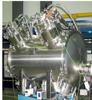
35-pole 4.2 Tesla, \lambda=60 mm superconducting wiggler for LNLS light source. 2009
