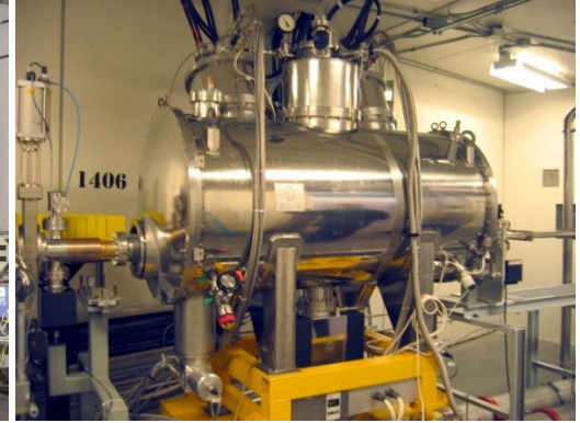
63-pole 2.2 Tesla, \lambda=32 mm superconducting wiggler for Canadian Light source. 2005
