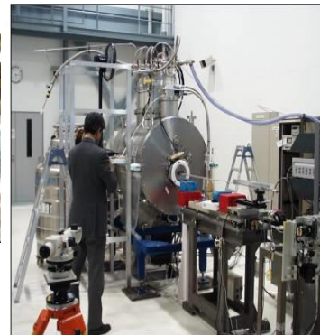
10 Tesla superconducting shifter for SPring-8. 2000
