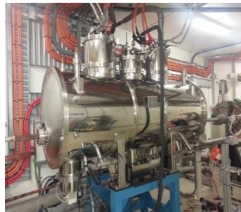
49-pole 4.2 Tesla, \lambda=52 mm superconducting wiggler for AS light source. 2012
