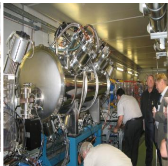
119-pole 2.1 Tesla, \lambda=30 mm superconducting wiggler for ALBA light source. 2010
