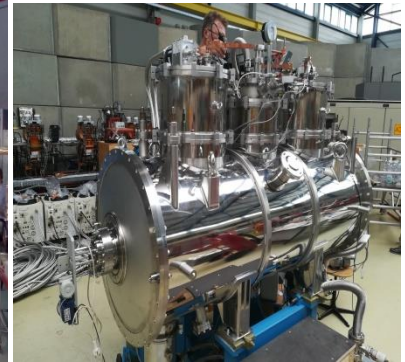
22-pole 7Ttsla, \lambda=125 mm superconducting wiggler for DELTA (Dortmund) 2019
