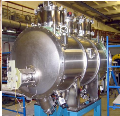
49-pole 4.2 Tesla, \lambda=48 mm superconducting wiggler for Diamond Light source. 2009
