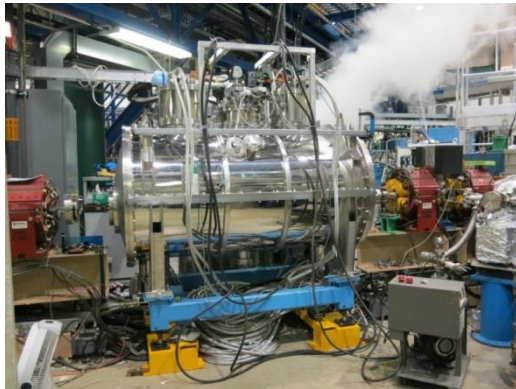
15-pole 7.5 Tesla, \lambda=198 mm superconducting wiggler for LSU CAMD light source (Baton Rouge) 2013
