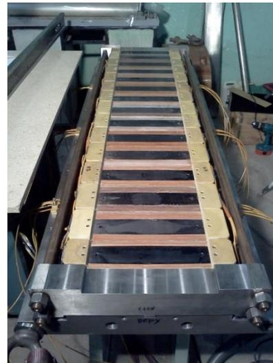
The installation of an insertion device with so high field at an accelerator working energy of 1.35 GeV is quite a complex accelerating challenge, as considerable effort was required for compensation of the influence of the magnetic field on the magnetic structure of the storage ring. All problems connected with the influence of the wiggler field on the beam dynamics were successfully solved during the wiggler commissioning with electron beam.
