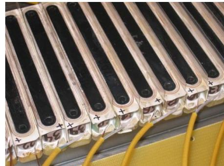
**High field long period superconducting multipole wigglers are used for production of hard X-rays on storage rings with low electron energy (BESSY 1.7 GeV, CAMD LSU 1.35 GeV, Siberia-2 2.5 GeV, Dortmund university 1.5GeV)**
