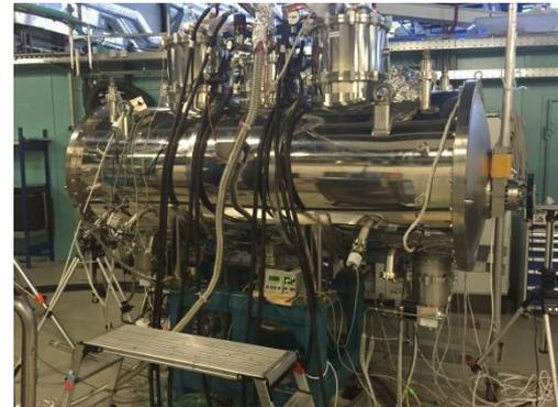
Indirect cooling system. Liquid helium used as cooling agent
