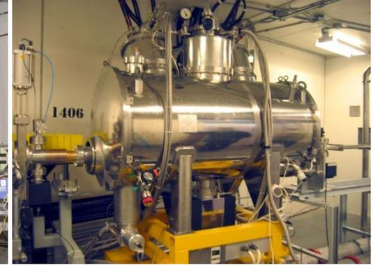
63-pole 2.2 Tesla,  $\lambda=32$  mm superconducting wiggler for Canadian Light source. 2005
