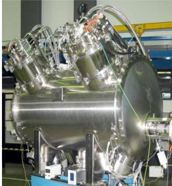
35-pole 4.2 Tesla,  $\lambda=60$  mm superconducting wiggler for LNLs light source. 2009
