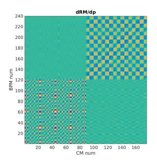
**FORM derivate** with respect to  $\delta p/p$ . Could be used to fit non linear fields.
