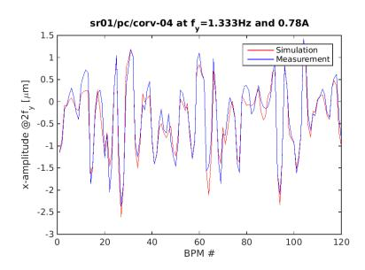
Amplitude of the  $2f_y$  line for the horizontal BPMs.
