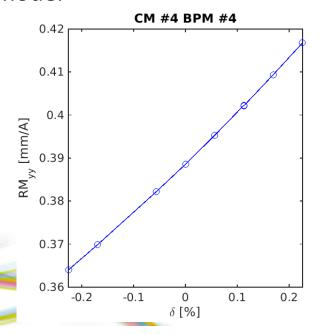
**FORM** element as a function of  $\delta p/p$  induced by a RF frequency change.
