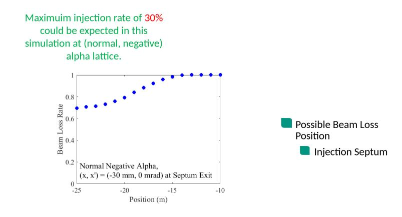
How to increase the injection rate? ... **Try to adjust exit angle at septum**
