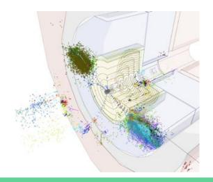
Jet tagging capabilities with 5TeV b-jets in FCC-hh, but using the CLIC software and the FCC vertex tracker, combined in the CLIC detector model
