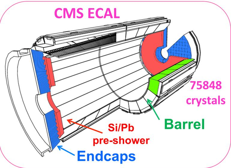
Crystal calorimeters require constant monitoring to correct for environment effects and radiation induced light output change, and periodic channel-to-channel calibration. Monitoring corrections are promptly computed and are available for prompt event processing. The full statistics of one year is used to compute the calibrations. A full detector calibration of the Run2 data (2016-2017-2018) was done during 2019 to achieve optimal performance.
