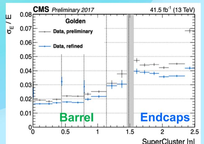
The Figure shows the achieved energy resolution for electrons versus the position in the detector. A large improvement is observed between prompt processing performance and new refined recalibration. The effect is particularly evident for the forward region, where an excellent response stability has been restored.
