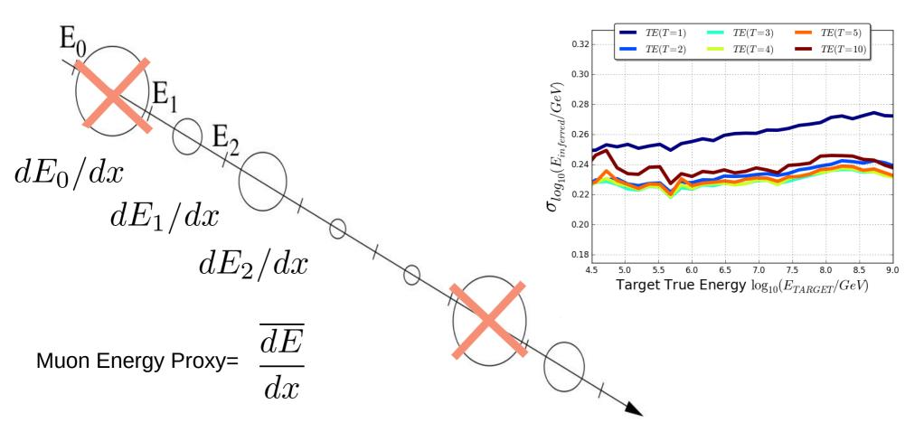
This is a simple version of Truncated Mean Energy Loss Rate<sup>1</sup> using the energy loss pattern. The complete version as used in the IceCube neutrino observatory accounts for detector effects ect.
