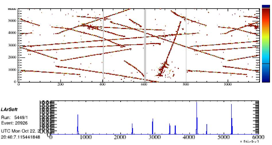
Remove bad hits, coherent noise, deconvolute, 2560x6000 12 bit
