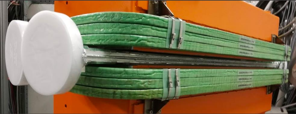
Two-way thin vacuum chamber (Aluminium): 25 mm gap
