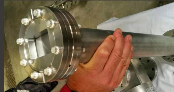
0.25 Beryllium window, separating with LINAC vacuum
