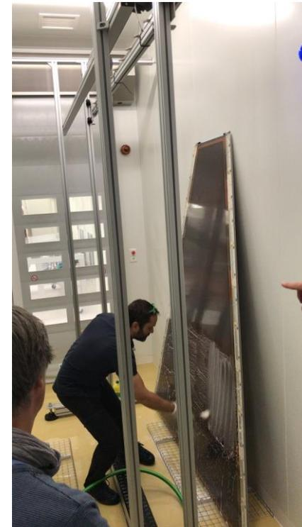
500x500 mm<sup>2</sup> resistive Micromegas produced for muon densitography (for Security, Cultural Heritage, and industrial applications). Screen-printing at a pitch of 500 μm on kapton now used at CEA to improve the resolution by charge sharing.
