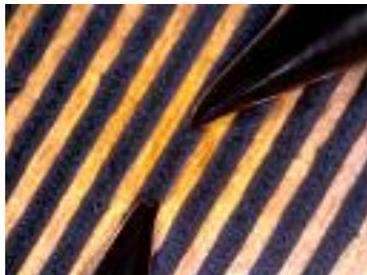
Resistivity measurement protocole defined and reproducible, using circular probe and square 'Ochi' probe for plain coating
