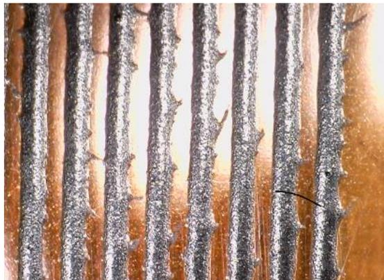
Solution : Discharge the base foil and work in a dust-free environment
