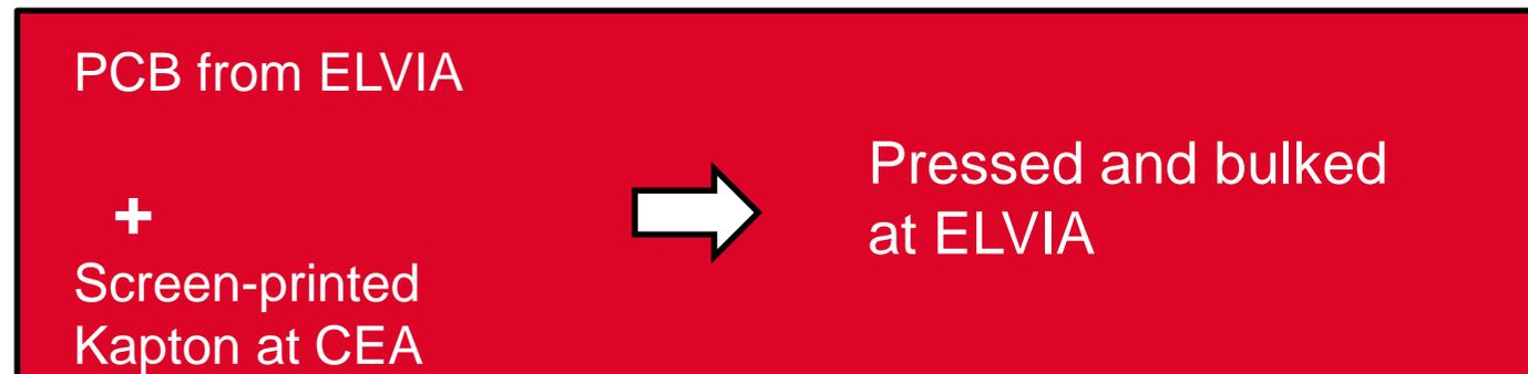
In 2018, 40 more resistive bulks will be produced at ELVIA, 20 with screen printing and 20 with DLC. Issues on pressing dispersion and stability, now understood: high resistivity past tends to crack when pressed
