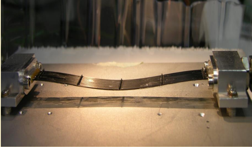
Deformation at 140 atm
