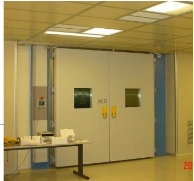
Environmental chamber - S.Piero lab Angelantoni WZH30-A1
