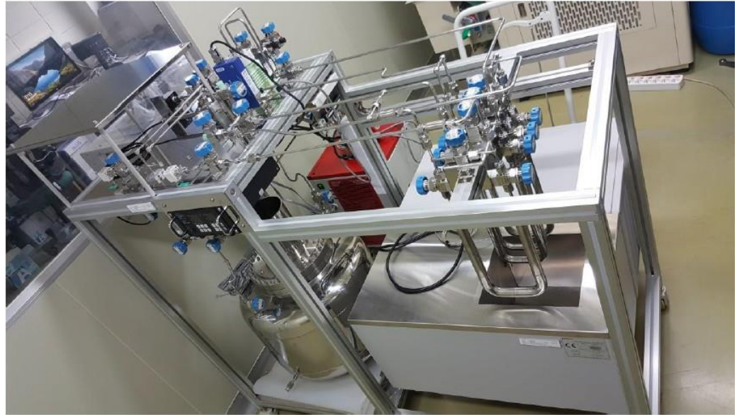
Assembled radon measurement device at SNU
