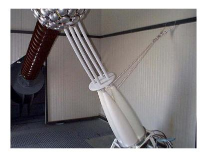
Oil transformer (test 400 kV) output bushing and line towards Alice's HVP +350 kV 135 kVA (used up to 75 kW)
