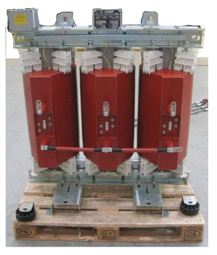
NIO1 resin transformer (courtesy M. Bigi and G. Serianni) rated 70 kV, tested 100 kV (NIO1 stays for Negative Ion Optimization phase 1, and its design voltage is 60 kV) M. Cavenago et al. "Precision HVP for ion mass analysis", Padua, 17 Sept 2019 7
