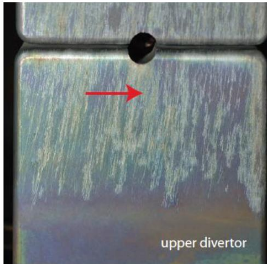
Arc trails on tokamak PFC. From Rohde 2010.
