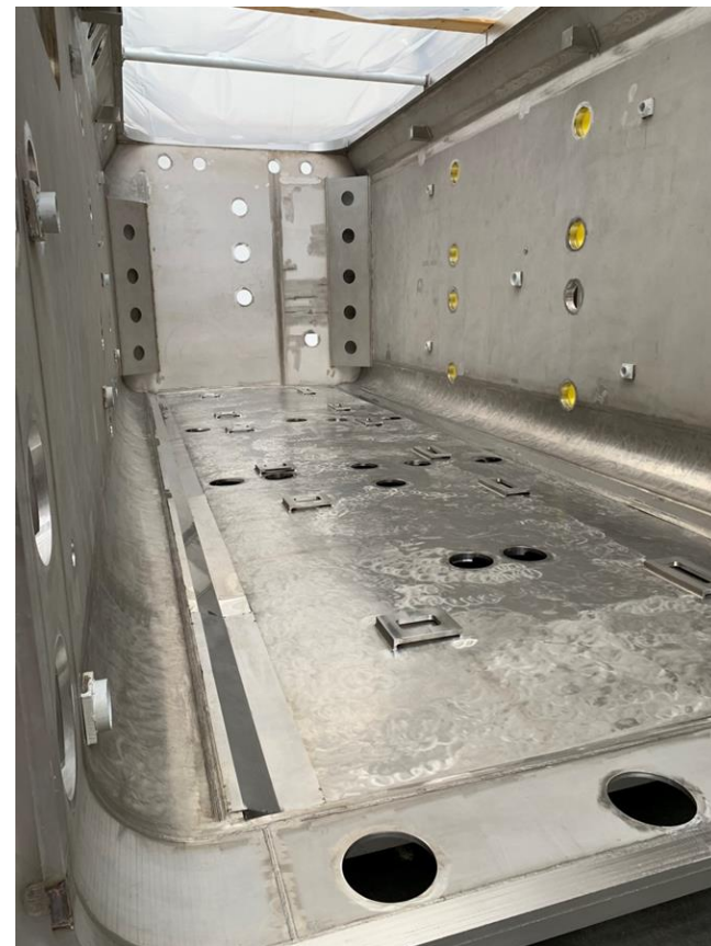
Beam Source Vessel (left) and Beam Line Vessel (right), during construction, both parts are made of AISI 316L stainless steel
