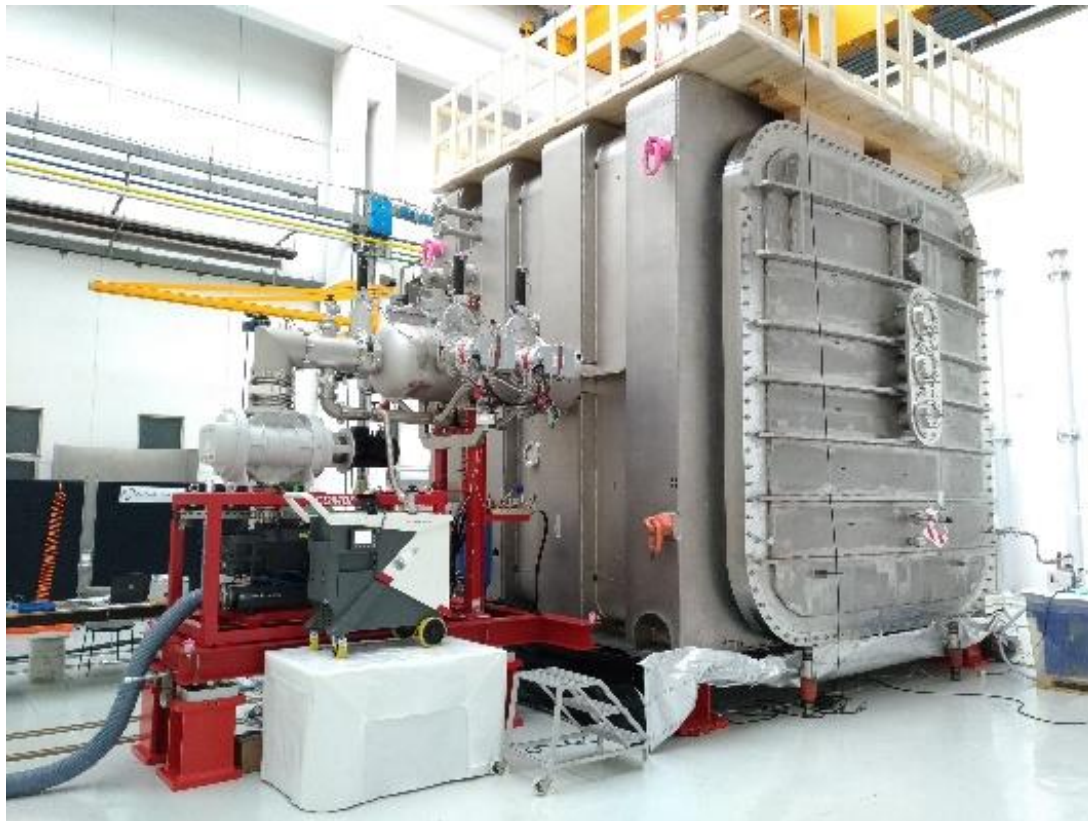
Beam Source Vessel (left) and Beam Line Vessel (right), during construction, both parts are made of AISI 316L stainless steel
