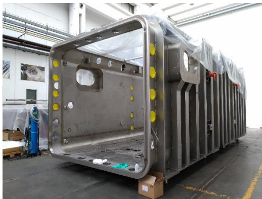
BLV in Feb 2019: welding of ports and other internal supports, before final machining
