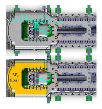
Lateral pumping of the accelerator helps a lot in reducing stripping losses inside the beam source
