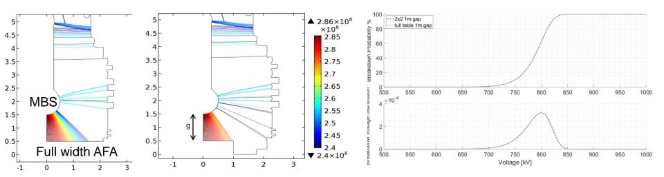
The most stressed part with 1m gap (worst case) is still between the MBS and AFA 1m radius AFA seems to be enough to characterize the V<sub>BD</sub> vs gap relation (same estimated breakdown probability)
