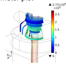
The -800kV water pipe is subjected to high electric field (5 kV/mm)
