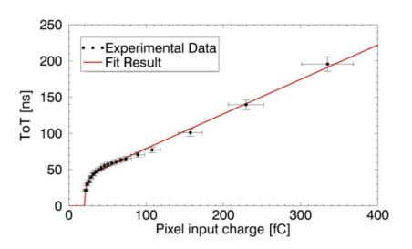
The length (in time) of these digital signals (the GEMINI output) is related to the input charge on the detector pad.
