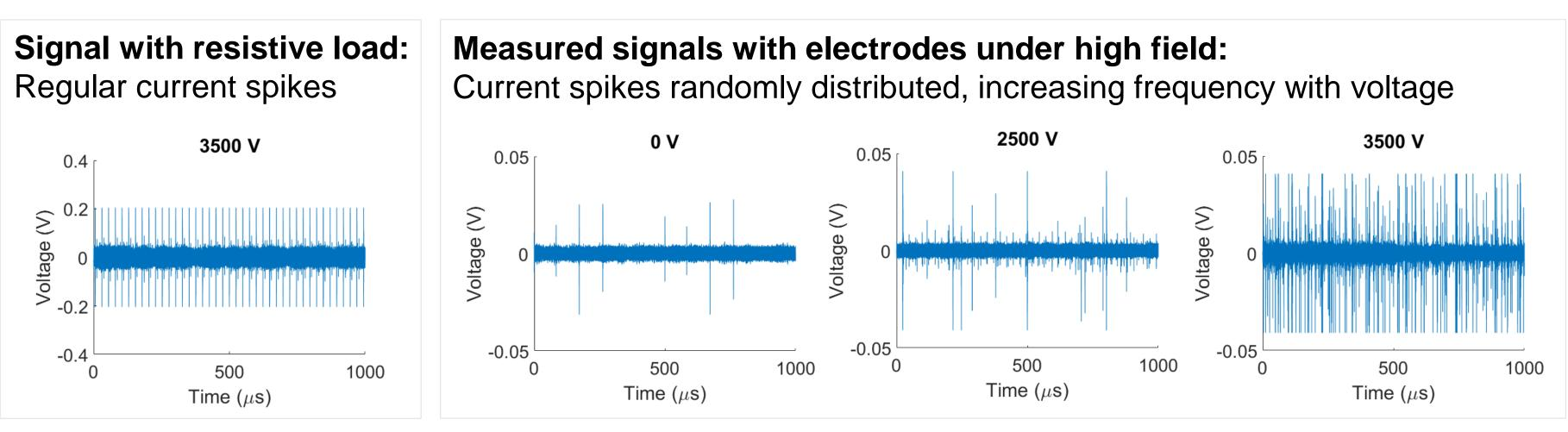
Measurements on the DC spark systems with a high voltage bias tee reveal voltage spikes and subsequent ringing. The ringing is believed to be caused by the dynamic response of the reactive elements in the high voltage power supply to an impulse of current.
