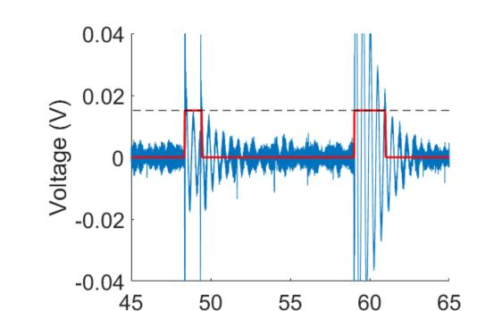
the voltage dependence of the time between impulses, strongly suggests that these are not external interference but related to field emission.
