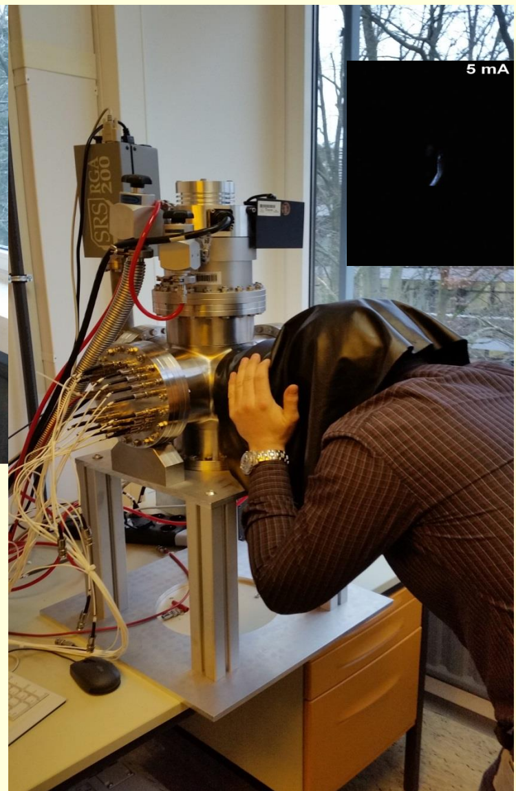
Figures: Observation of glow discharges during FE measurements
