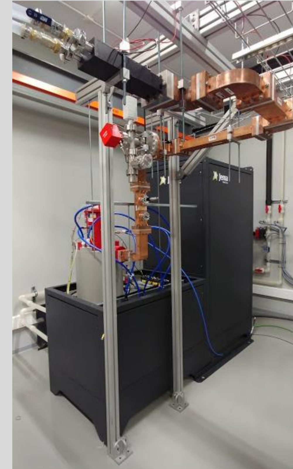
First modulator, klystron and waveguide network at the IFIC laboratory
