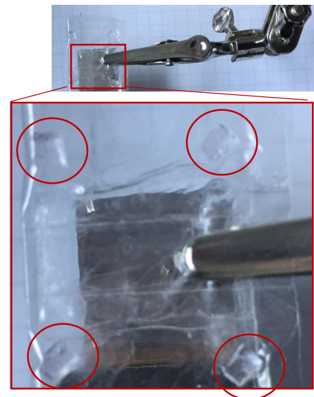
Reconstruction of position of 4 ^{133}\text{Ba} gamma sources (356 keV)
