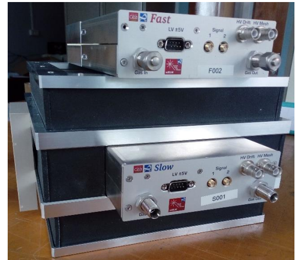
Assembly of a fast and a slow detector size ≈ 20 × 25 × 25 cm 3 (~14 kg)
