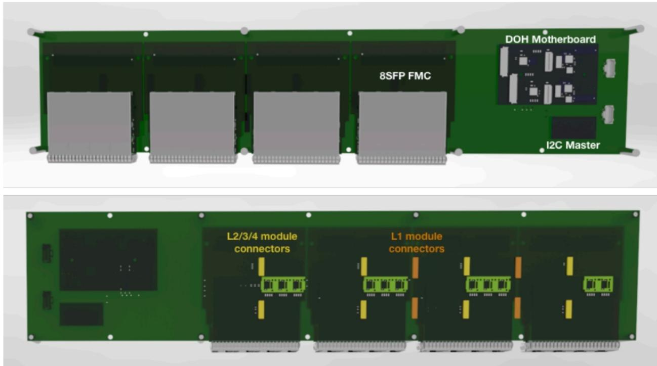
The [motherboards](#) of the CHROMIE telescope. The top image is the front of the board with the 8SFP FMCs, DOH motherboard, I<sup>2</sup>C master, and power and bias connectors. The bottom image shows the back of the board with the module connectors. Design by Cerntech Ltd., rendering with KeyShot.
