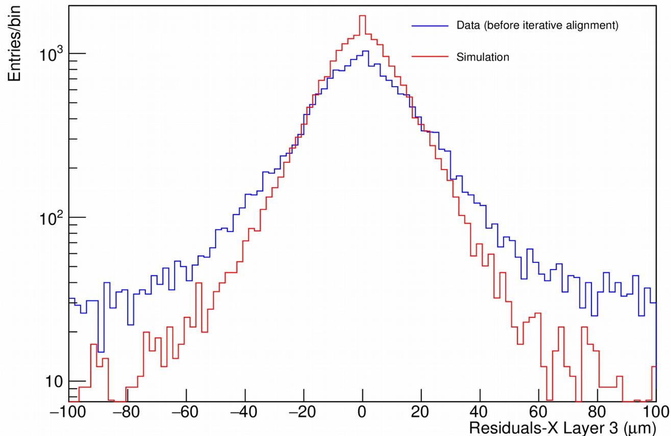
**X-residuals** for the left module of Layer 3 for a **120 GeV  $\pi^+$**  beam (comparison between beam test data before iterative alignment and simulation). Simulation residuals scaled for **26814** valid tracks from the beam test run out of **32536** total events. Standard deviation (beam test): **29.1  $\mu\text{m}$** . Standard deviation (simulation): **19.8  $\mu\text{m}$** .
