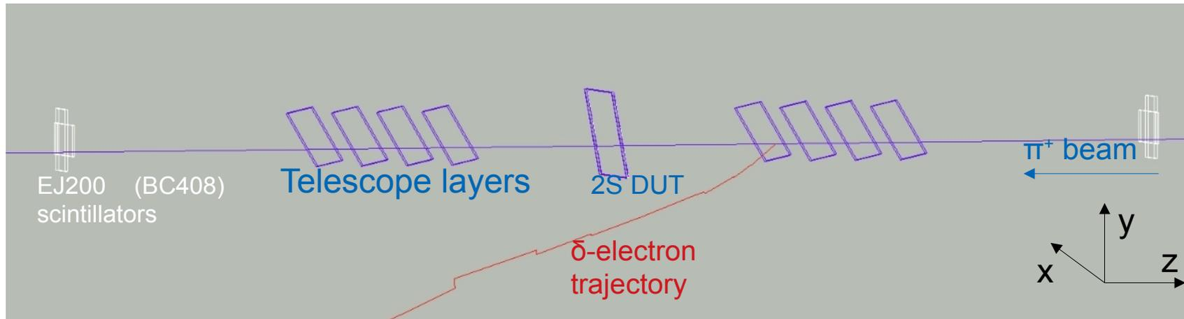
The DUT is a **2S** module: 2 Si sensors (**102700  $\mu\text{m}$  X 94108  $\mu\text{m}$  X 320  $\mu\text{m}$** ), with spacing between the sensors: **2 mm**; strip pitch: **90  $\mu\text{m}$** ; active depth: **240  $\mu\text{m}$** .
