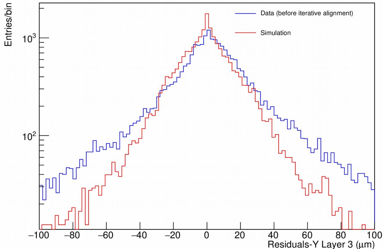
**Y-residuals** for the left module of Layer 3 for a **120 GeV  $\pi^+$**  beam (comparison between beam test data before iterative alignment and simulation). Simulation residuals caled for **26814** valid tracks from the beam test run out of **32536** total events. Standard deviation (beam test): **31.4  $\mu\text{m}$** . Standard deviation (simulation): **23.3  $\mu\text{m}$** .
