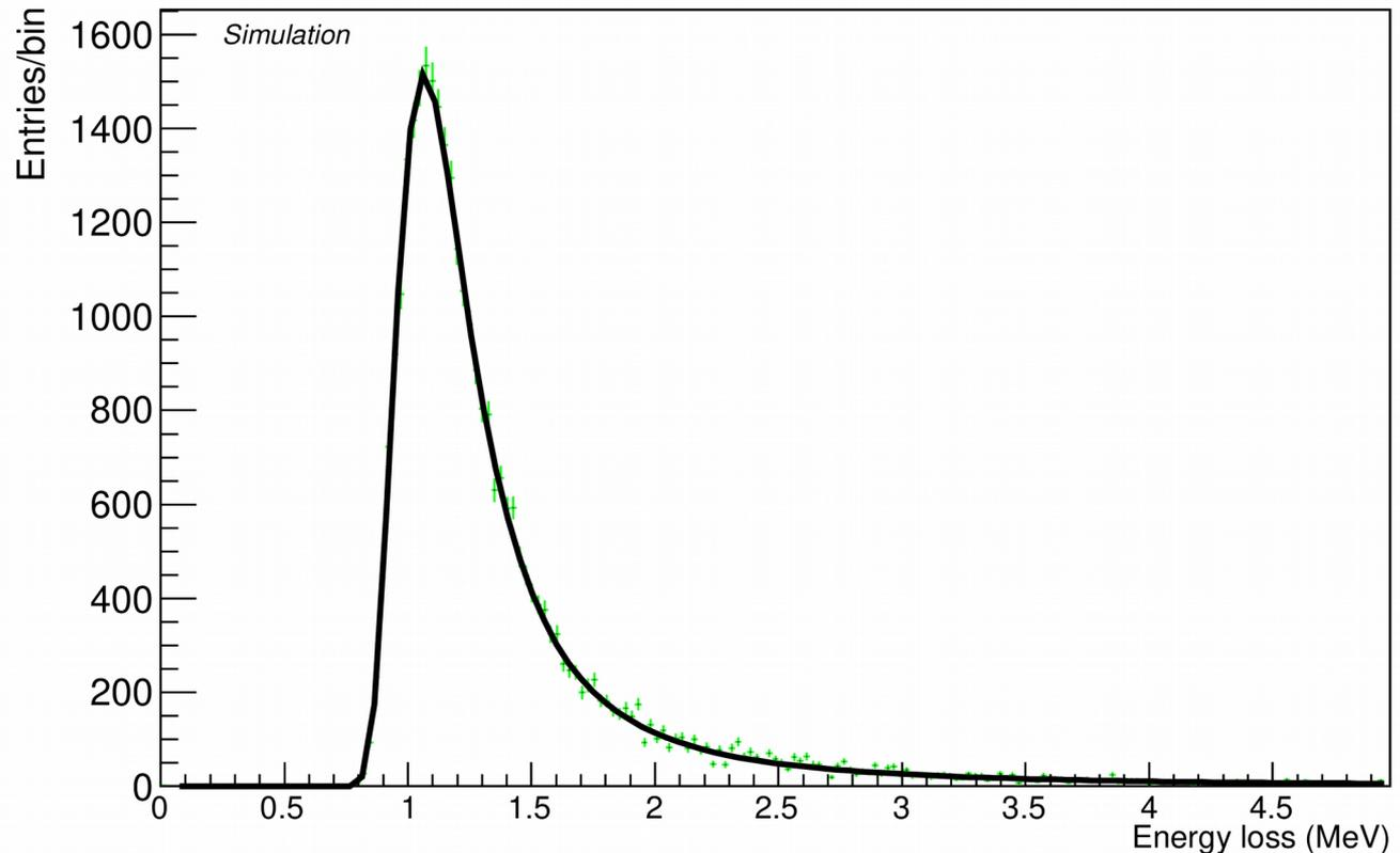
Total energy lost by primary particles (120 GeV  $\pi^+$ ) in CHROMIE layer 1 after a Landau fit (simulation).
