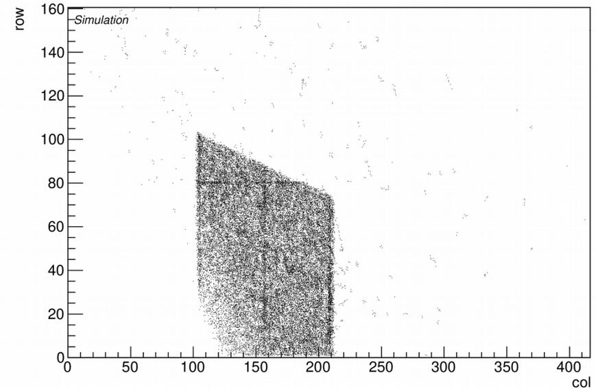
Cluster occupancy per column per row for the left module of Layer 2 for a 120 GeV  $\pi^+$  beam (left: beam test, right: simulation simulation with beam diameter = 15 mm and  $\sigma_E = 100$  keV); the beam size was measured from the beam spot on the cluster occupancy map for the same module, obtained from the analysis of the real run, and thus the above parameters were selected for the simulation run).
