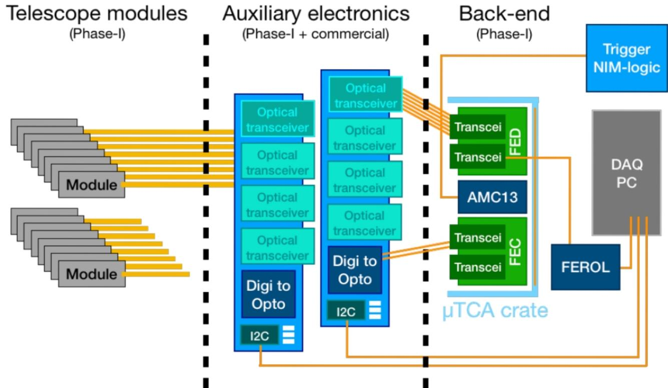
The, mostly CMS standard, [readout](#) and [DAQ](#) of the CHROMIE Telescope. It is analogous to the readout of the [CMS Phase-1 Inner Tracker readout](#). The yellow ribbons and black arrows represent [electrical](#) links. The orange arrows represent [optical](#) links.
