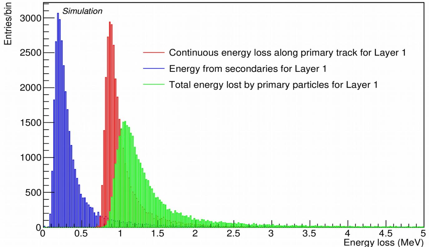
Energy lost by primary particles (120 GeV  $\pi^+$ ) in CHROMIE layer 1 (simulation).
