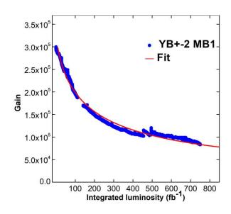
Effects of prolonged exposition to radiation: •loss of gas gain •rise in spurious signal rates ("dark rate") •increase in leakage currents ("dark current") •development of self-sustained discharges set off at high radiation rates (Malter effect)
