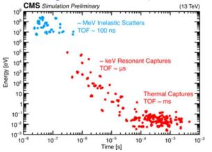
Energy of simulated neutron vs. time since pp collision for hits in the CSCs, with GEANT4 simulated minimum-bias pp collisions at 13 TeV
