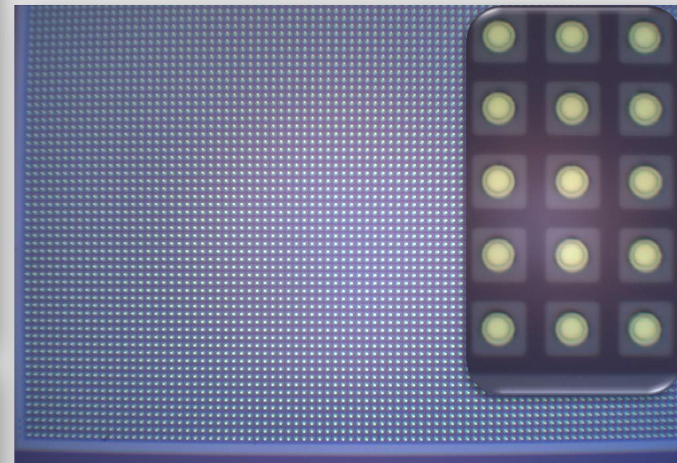
Pitch - 50 \mu\text{m} , strip width - 25 \mu\text{m}
