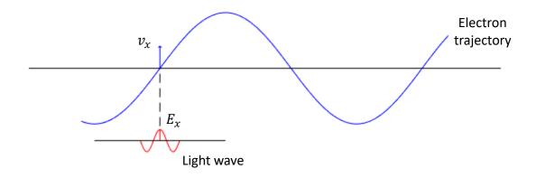
2) Electron velocity and electric field in opposite direction => electron gains energy
