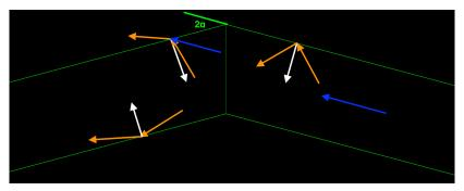
An optical photon travelling parallel (blue) to the 1st tile ( $\theta_{inc} = 90^{\circ}$ ) will be mapped by the rotation  $\alpha$  into a photon with  $\theta_{inc} = 90^{\circ} - 2\alpha$  in the 2nd tile.
