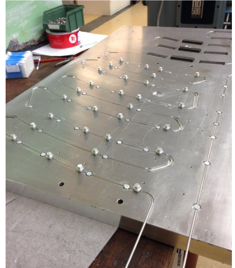
Gluing jig for pipes, inserts and carbon foam
