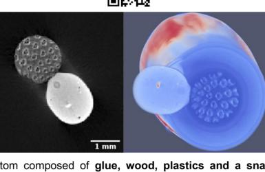
Left: photo of the phantom composed of glue, wood, plastics and a snail shell. Middle image is an axial slice showing the wooden toothpick with its microstructures and the glue with some small air pockets and dense material. Right image is a volume rendering of the reconstructed CT slices, the colour scale here represents the CT number (density).
