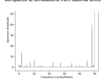
Left: This spectrum amplitude splits the frequency components of the beam intensity for one measurement. It shows that there is a high amplitude 2 Hz component and a relatively lower amplitude 50.0 Hz component. 50.0 Hz is the mains frequency in the UK and so this is very likely to be directly related. The 2 Hz component is unknown, it is currently hypothesised to be related to the RF power to the dees of the cyclotron or the
