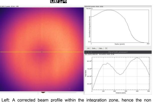
uniformity in the centre of the detector. The ROI selected is both radially summed (top right) and a line profile is calculated (bottom right). These can be compared to simulations from Jacinta directly.
