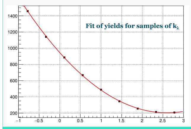
Approach to model anomalous  $k_{\lambda}$  signals in **COMBINE** (counting experiment,  $k_{\lambda}$  is a POI): yield parametrized vs  $k_{\lambda}$ with **quadratic function** by fitting various  $k_{\lambda}$  samples after the full selection.
