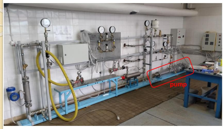
The pressure head up to 2.5 MPa in the installation is induced by a progressive cavity pump with variable speed operation. The water mass flow rate in the circuit is adjusted by changing the rotational speed of the pump in the range 10–60 Hz. Two bypasses of the pump with different diameters enable precise adjustment of small mass flow rates
