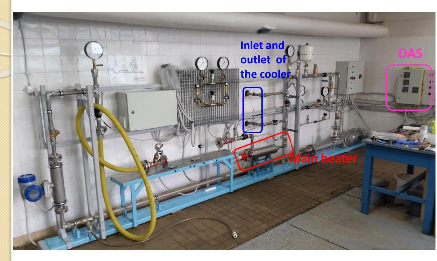
The main heater and the air flow cooler enable adjustments of the water temperature in the circuit in the range from room temperature to about 70°C. DAS includes four 8-channel data recorders.
