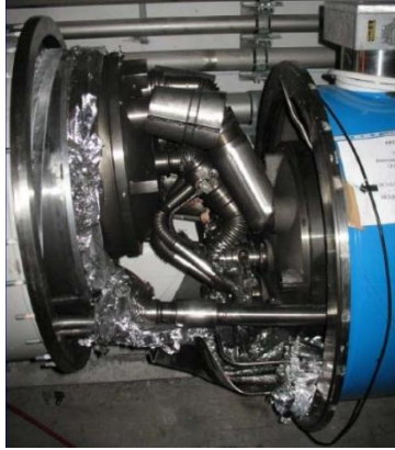
This is the result of a chain of events triggered by a quench in an LHC bus-bar
