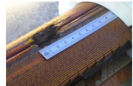
This is the result of a quench in the pre series magnet during its qualification test
