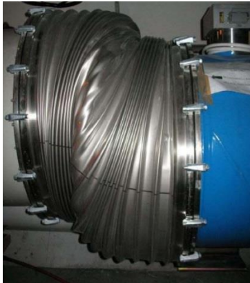
This is the result of a chain of events triggered by a quench in an LHC bus-bar
