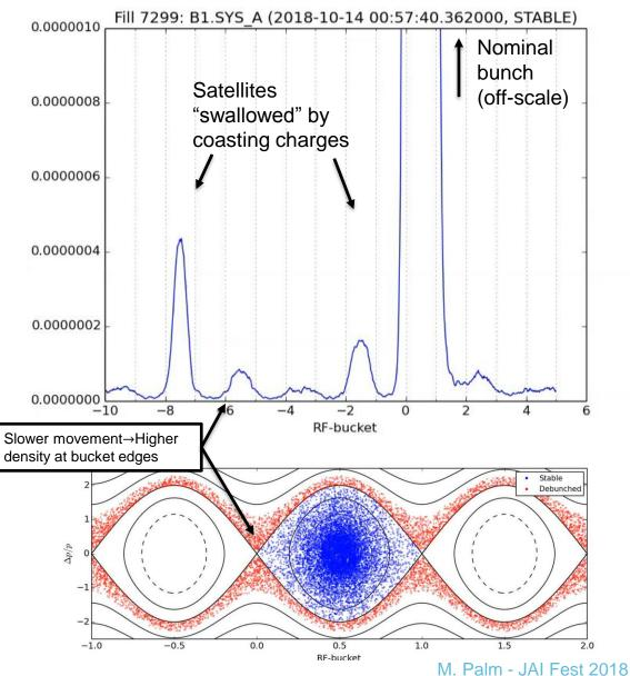
□ RF-problem during vdM-scan October 2018 ⇒ Continuous "leakage" from filled buckets  $\Rightarrow$  Debunched protons coasting around ring 5h time-lapse of BSRL
