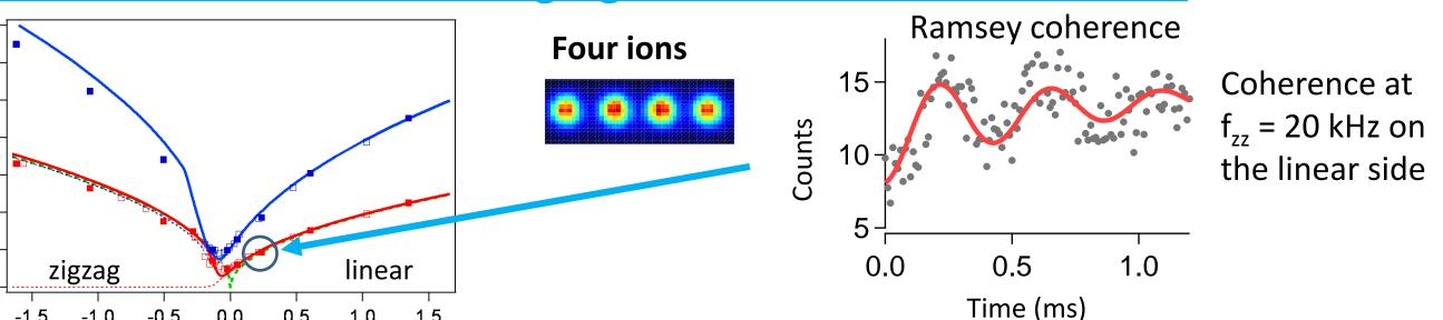
Motional heating of the zigzag mode and Ramsey coherence are being investigated near the transition to understand decoherence properties of the order parameter and short term trap noise.
