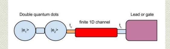
The effect of the channel + lead on the TLS can be incorporated into an effective TLS Hamiltonian.
