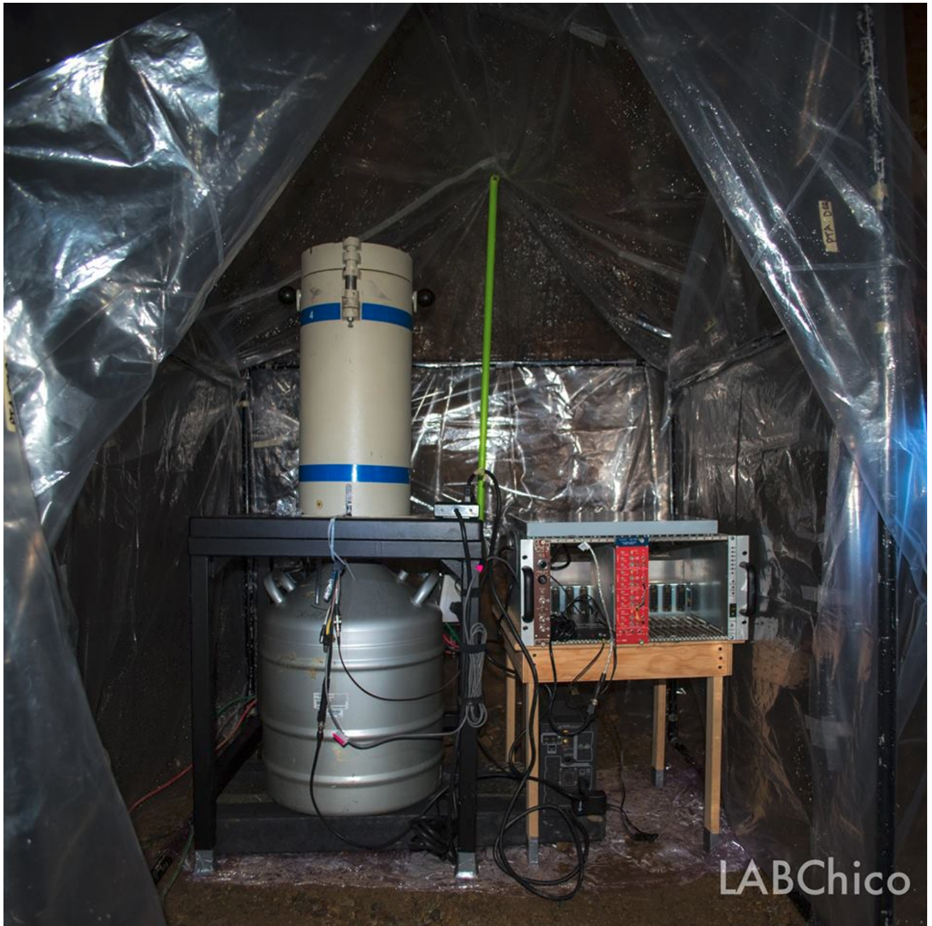
Complete installation of the detector, shielding and electronics inside the leak-proof tent.
