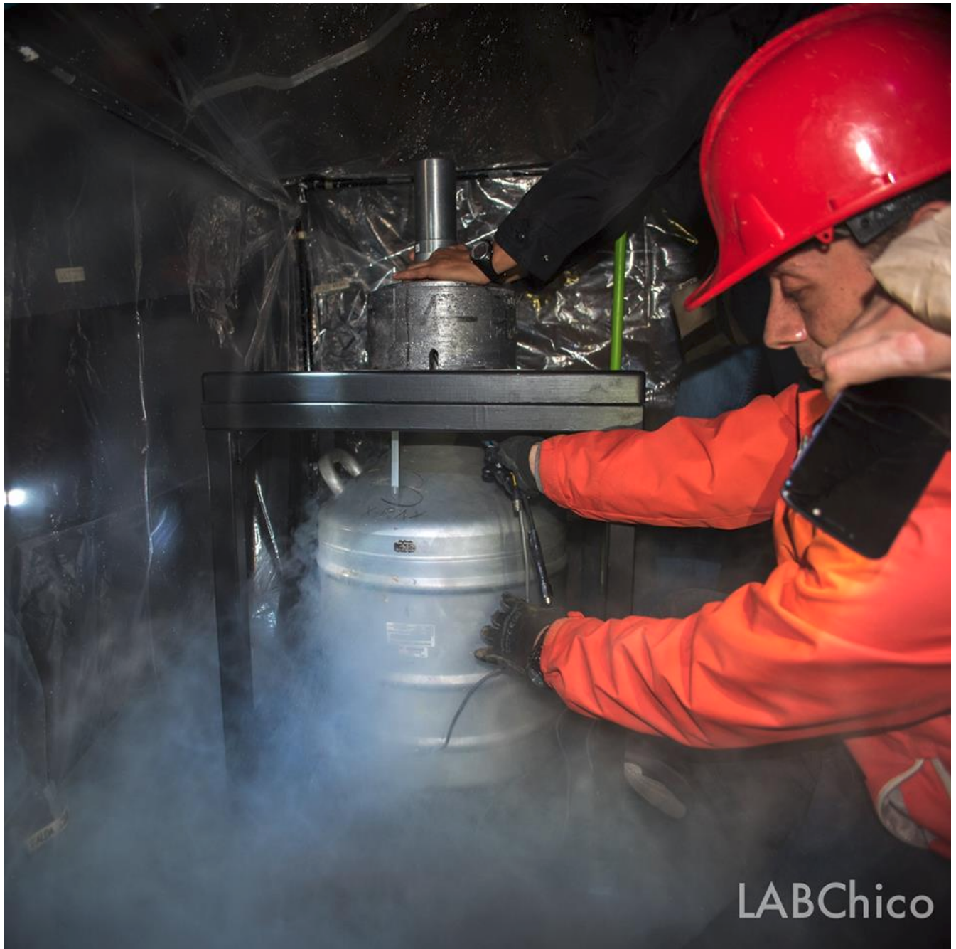
Dr. Alexis Aguilar Arévalo inserting the HPGe detector into the LN2 dewar.
