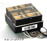
The MCP-PMT XP85012 with 64 anode pads is transformed into the 4-channels detector by merging 16 pads (4 × 4) of each cell into a single channel
