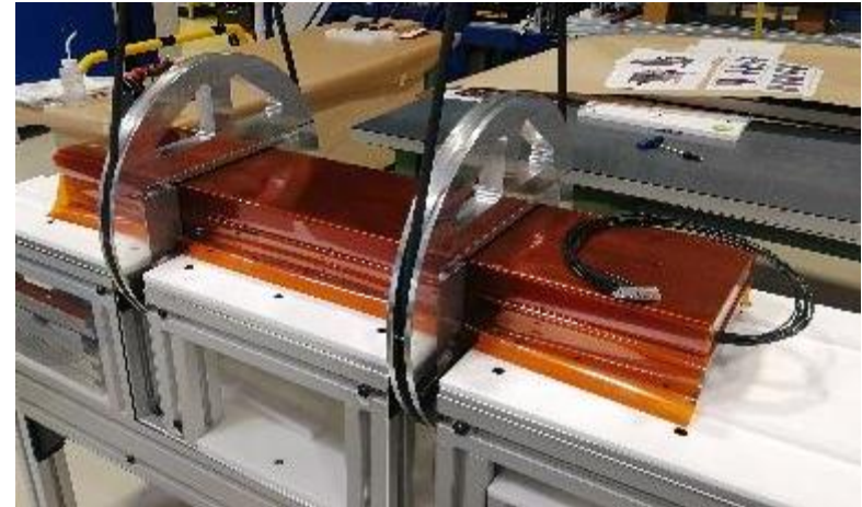
Coil rotation tooling and ground insulation
