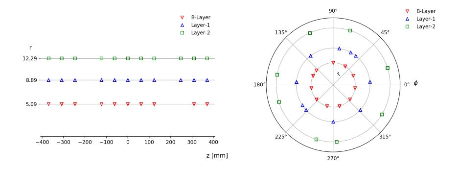
• The positions of modules in  $\varphi$  and r on the barrel layers
