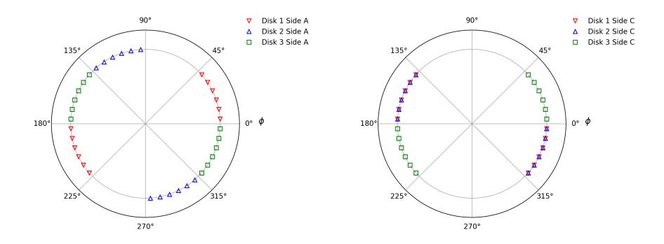
• The positions of modules in  $\varphi$  on the disks on side A (left) and side C (right). The modules on each disk are centered at a radial distance of 119.2 mm.
